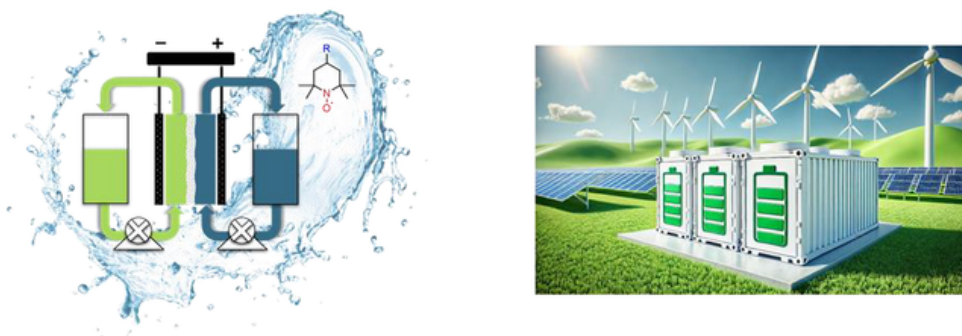
Figure 1. Nitroxide-based aqueous organic redox flow battery for renewable energy storage.
